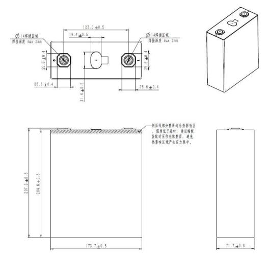
Fig. 15 Diagram of cell size and appearance 图 15 电池尺寸及外观图
